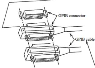
Total cable length: Up to 20 m Cable length between devices: Up to 4 m Number of devices that can be connected: Up to 15
