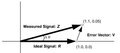
The modulation accuracy is described simply using the diagram above.
