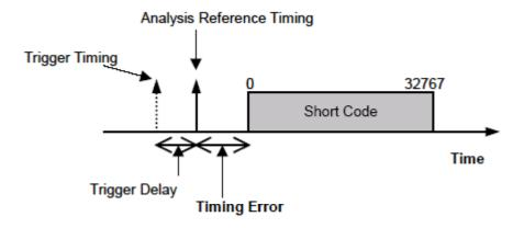
The analysis reference timing is the triggering timing with External Trigger plus the Trigger Delay. The short-code starting position is searched for by internal analysis and the difference between this position and the reference timing is represented in 64\*N (chips) and the fraction is represented in time resolution (0.01 µsec).
