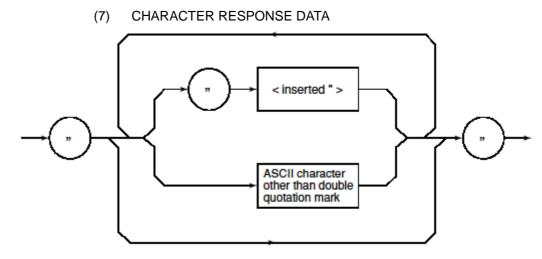
String response data is transmitted as an ASCII character enclosed with double quotation marks.
