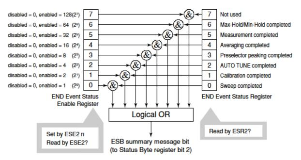
The END Event Status Enable Register is used to select which bits in the corresponding Event Register will cause a TRUE summary message when set.
