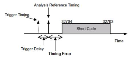
If Pilot PN Sequence Offset is 64 chips, the short-code starting position is shifted 64 chips; that is, it has a pattern starting at 32704, passing 0, and ending at 32703. In this case, for Pilot PN Sequence Offset of the transmitter tester, set Analysis Start to 64 chips. Thus, Timing Error is calculated assuming that Pilot PN Sequence Offset is 64 chips.
