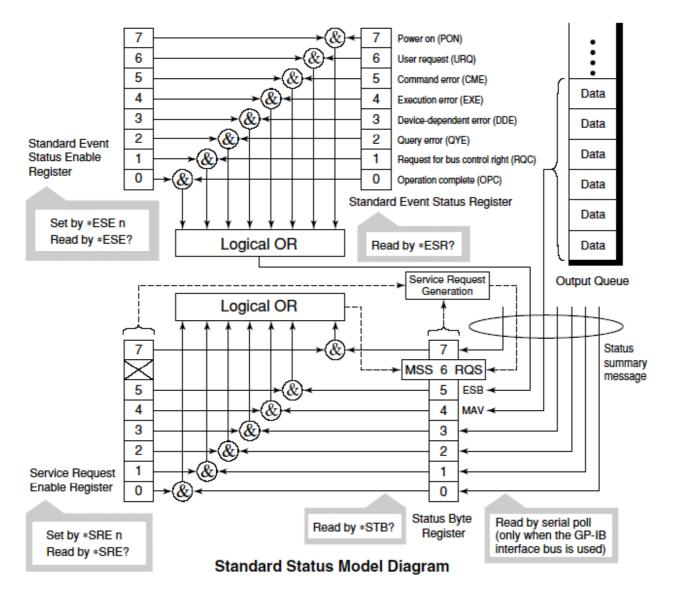
The diagram below shows the standard model for the status data structures stipulated in the IEEE488.2 standard. In the status model, IEEE488.1 status bytes are used for the lowest grade status. This status byte is composed of seven summary message bits from the higher grade status structure. To create these summary message bits, the status data structure is composed of register and queue models.
